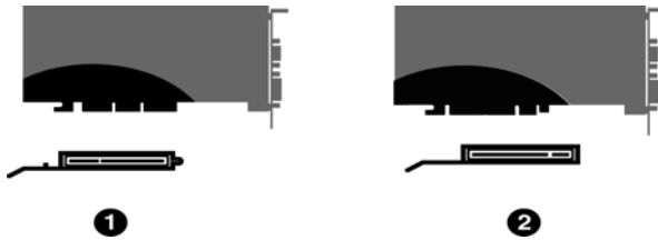
AGP and PCIe™ graphics cards and system bus connectors
